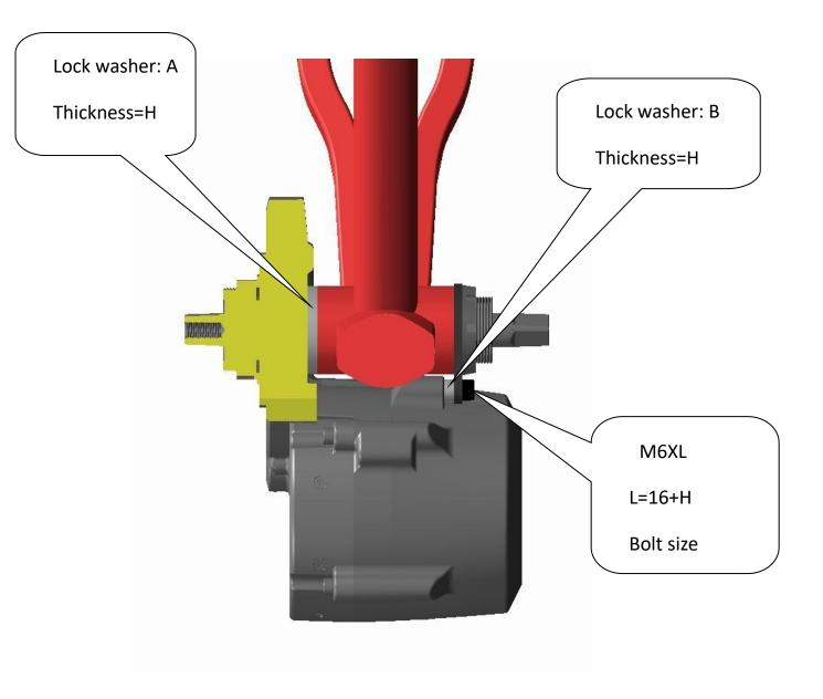
Note: the thickness H of lock washer A and lock washer B must be equal
